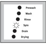
To select **Drain** press the **"Skip"** button three times, the **wash - rinse - spin** LED,s go out.
